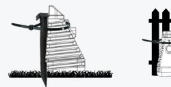
Secure to ground utilizing zip ties through the loop on the trap. Wrap zip ties around wood or plastic stakes & secure to fence posts or shrubs.
