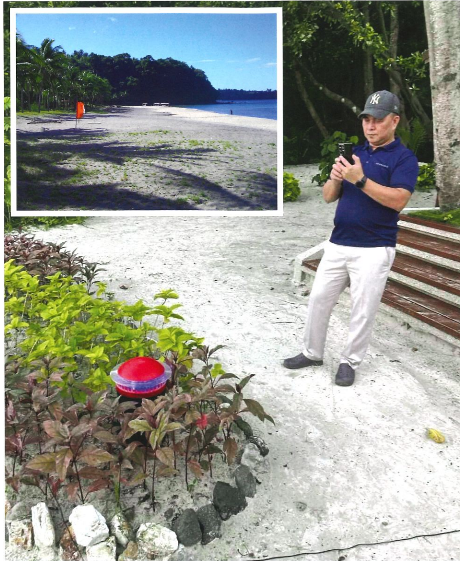
Light-based sandfly trap being tested outdoors. Inset: wet beach sand often acts as a breeding ground for sandflies in S E Asia.
