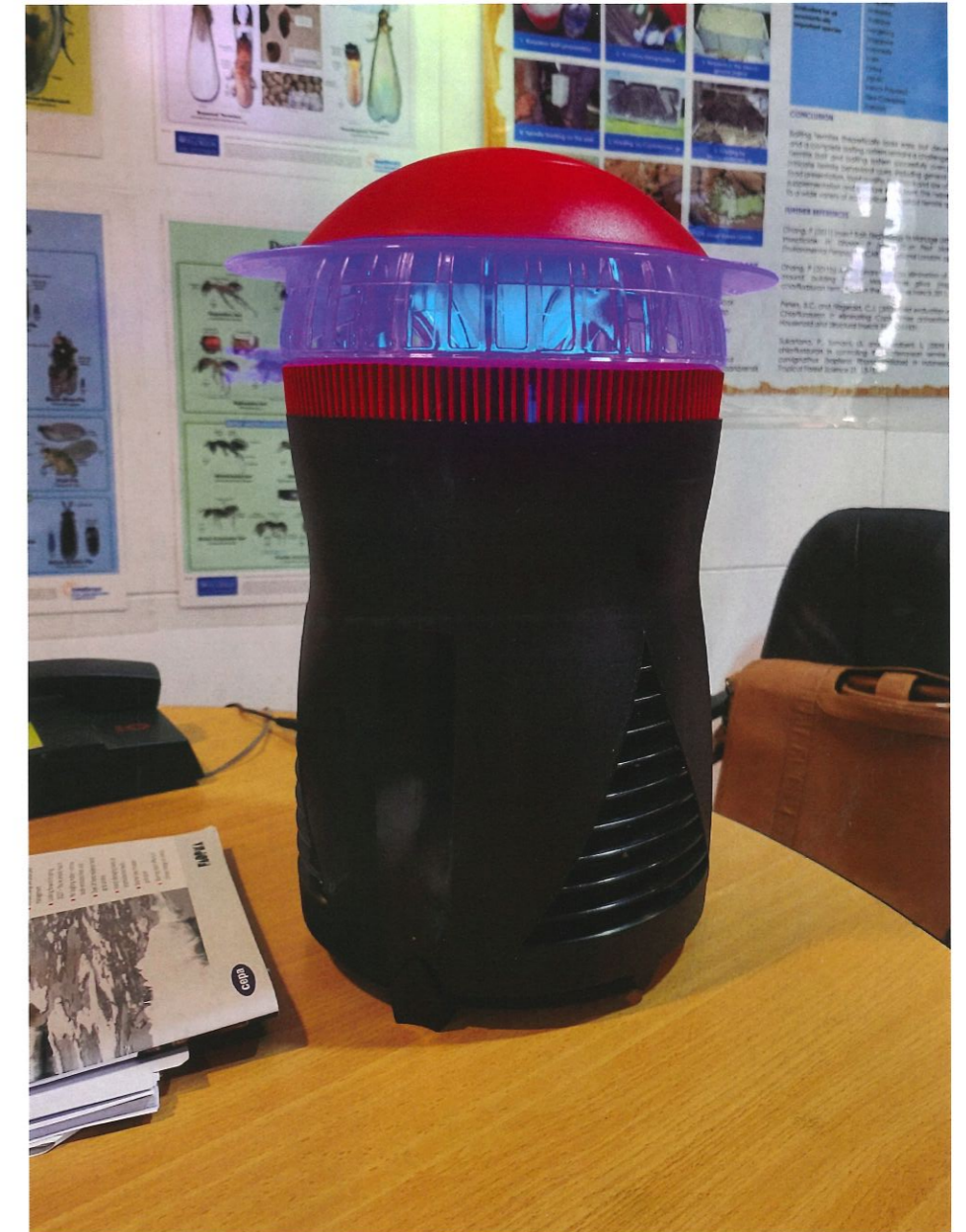
The light-based sandfly trap
